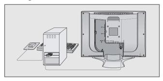
1 Connect the »VGA« socket on the television set and the appropriate socket of the PC using a VGA cable.
